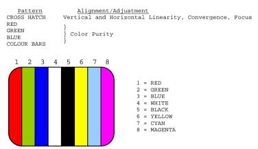
The color bar pattern is also analyzed to detect color RAM faults. If Color RAM Test 4 indicates no faults, a double-width band, half width bands, transposition or missing bands indicates a fault in 2E, 1C, or 2C chips.
